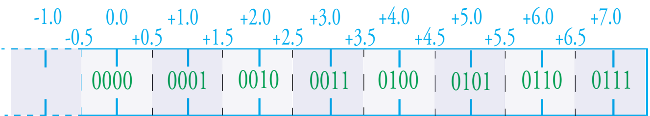
Figure 3.7.5 Enlargement of a measurement ruler that encodes sampled waveform height using 4 bits
