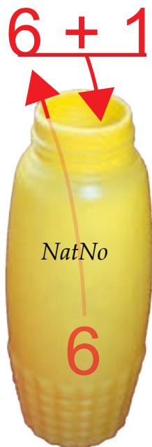
Figure 2.2.4 shows the value 6 stored in variable NatNo, being copied then added to 1 and the result 7 about to be stored
