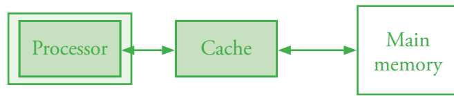
Figure 4.5.3.6 Cache memory situated between processor and main memory
