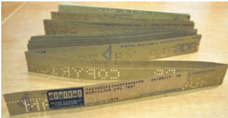
Figure 4.5.1.3 Paper tape used to store data and computer programs in the 1950's
